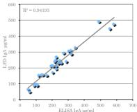
The SOMA sIgA LFD correlates well with values measured on the laboratory ELISA and when run in duplicates usually has within assay cvs of below 10%. Thus the test is accurate and reliable and easily performed in wide range of environments, away from the lab. Each batch of strips manufactured use their own specific calibration curve, uploaded to the SOMA LFD Reader.
