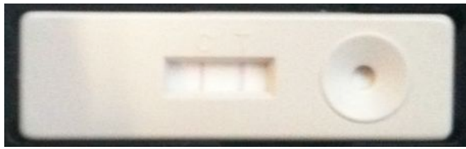
The IPRO LFD showing both the Control and Test Line
